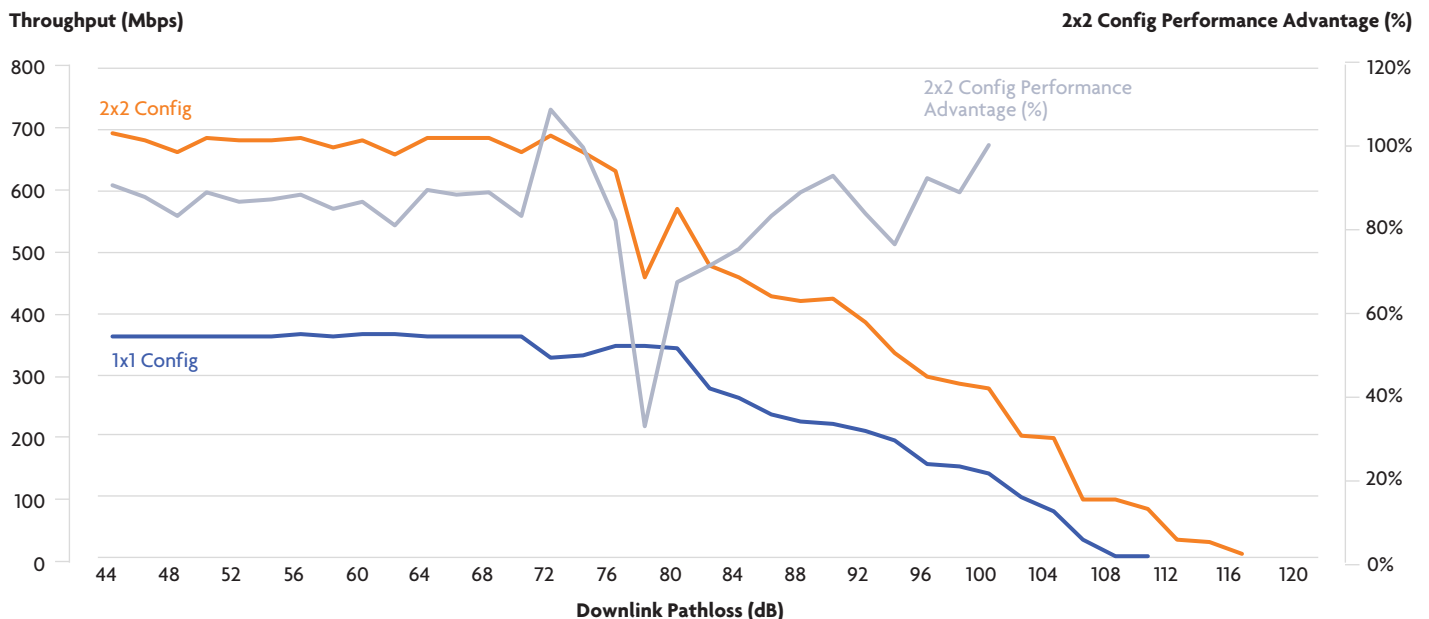
Figure 1. Throughput as a Function of Downlink Pathloss – 2x2 versus 1x1 antenna configurations (Test 65-66)
