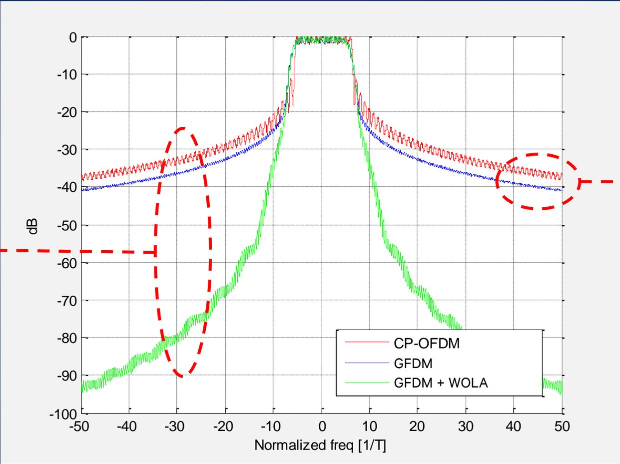
Time-domain windowing (like WOLA) significantly reduces OOB leakage
