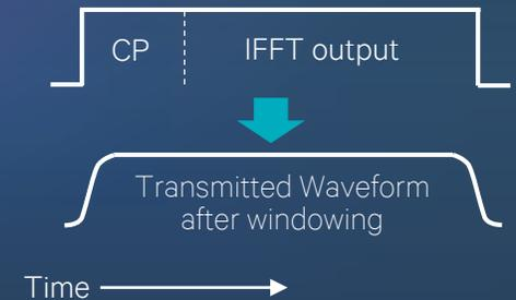
OFDM-based waveforms are the foundations for LTE and Wi-Fi systems today
