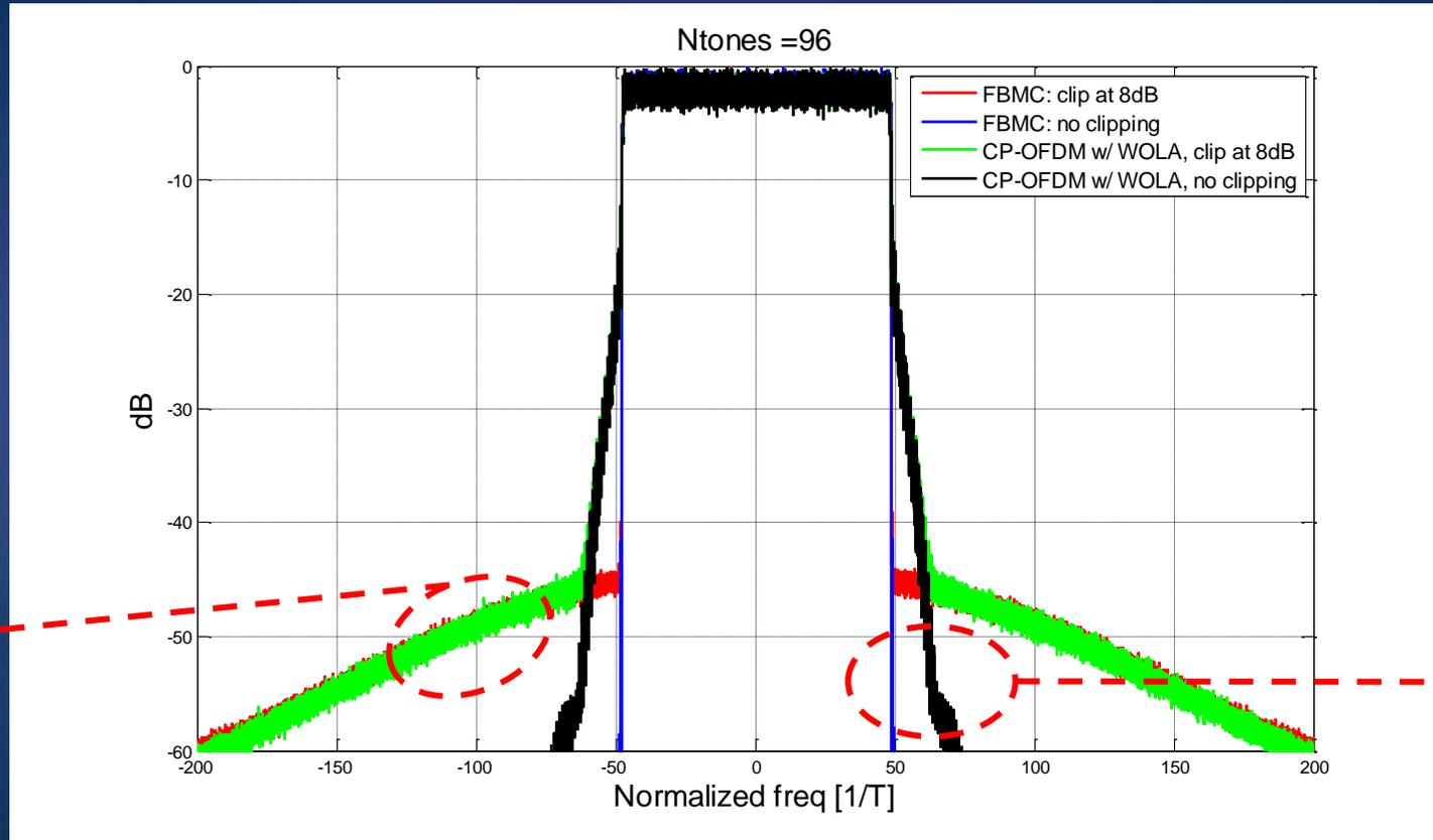
OOB leakage suppression performance reduces with PA clipping
