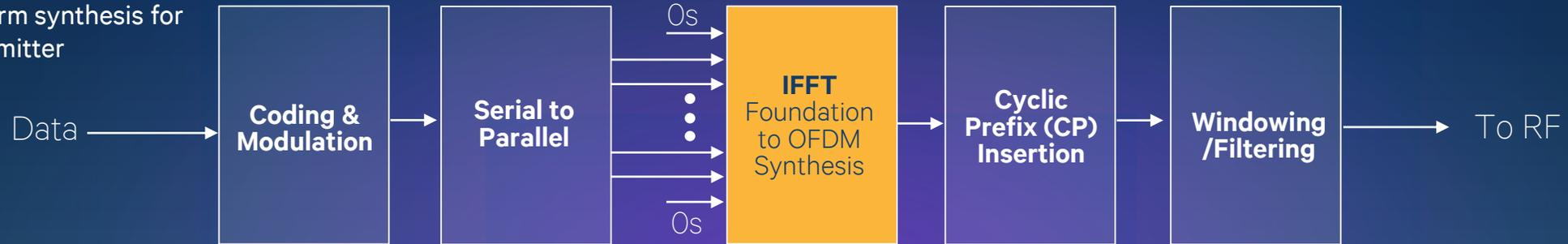
Data transmitted via closely-spaced, narrowband subcarriers – IFFT operation ensures subcarriers do not interfere with each other
