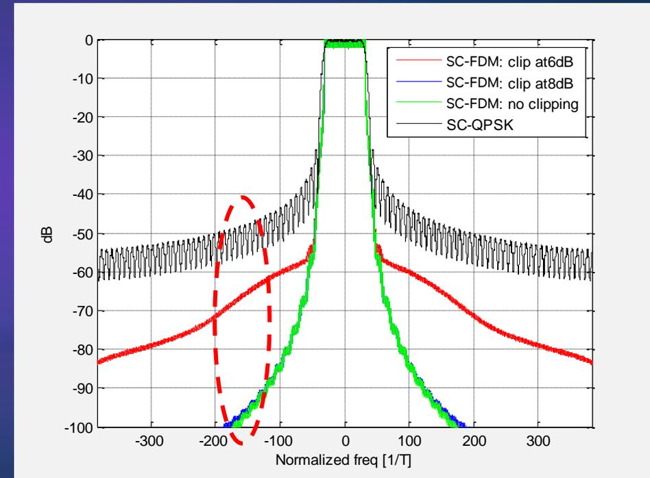
Significant improvement to OOB leakage performance using time-domain windowing (WOLA)
