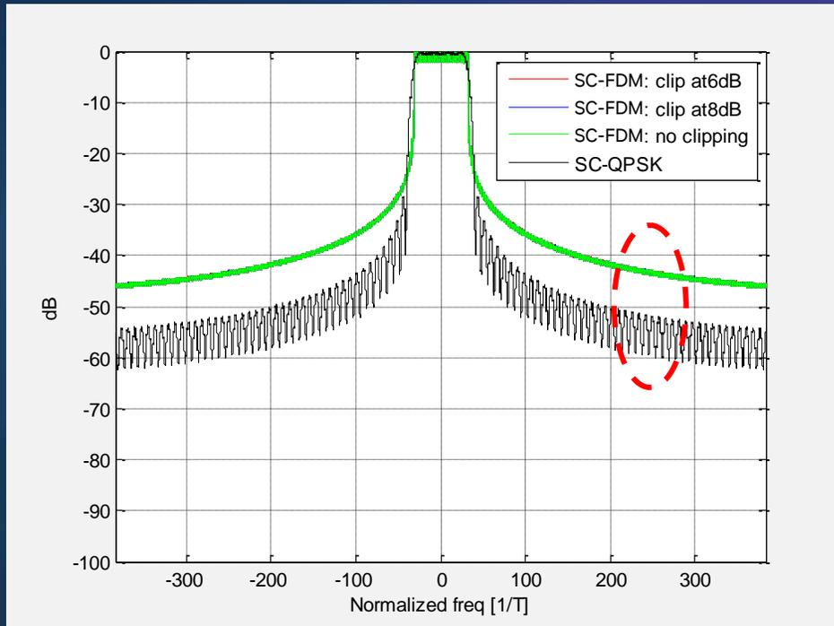
Higher OOB leakage than SC-QPSK due to discontinuities between OFDM transmission blocks
