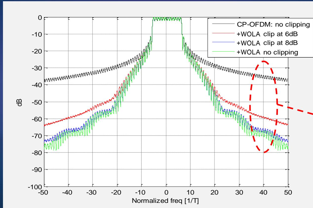
WOLA substantially improves CP-OFDM OOB leakage performance
